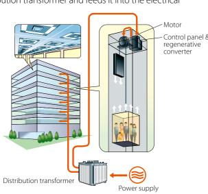
network in the building along with electricity from the power supply. Compared to the same type of elevator without a regenerative converter, this system provides an energy-saving effect of approximately 35%.\* In addition, the regenerative converter has the effect of decreasing harmonic currents.
