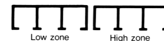
Two banks, in-line arrangement. Inconvenient because of confusion as to the dividing point.
