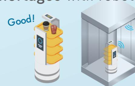
Coordination between elevators and robots assists robot operations so that the robots can move freely between floors in the building. It enables 24/7 security surveillance, delivery and cleaning independent of the availability of service personnel.
