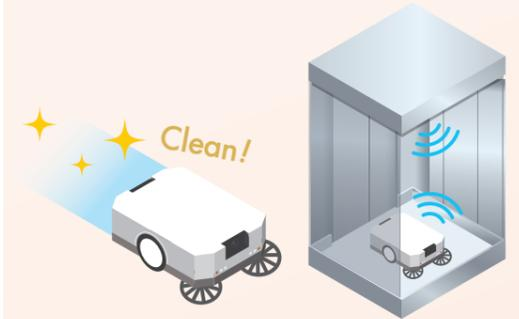
Coordination between elevators and robots assists robot operations so that the robots can move freely between the floors in the residence. It enables 24/7 security surveillance, delivery and cleaning independent of the availability of service personnel.
