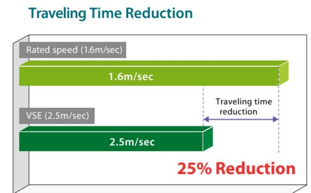
Traveling time can be reduced by approximately 25% when the elevator travels from the bottom to the top floor directly under rapid mode in VSE.
