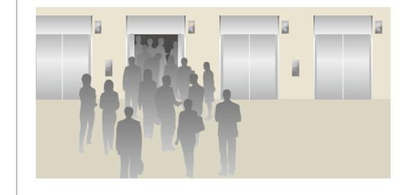
If a fully loaded car leaves a floor, a hall call is registered automatically.
